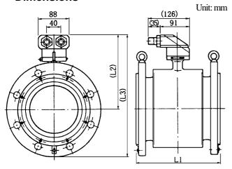
Figure 3. Detector Dimensions for Meter Sizes 150 mm (6") and 200 mm (8")
